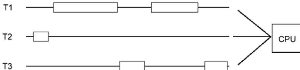
Figure 2-6. Three Threads Running Concurrently on One CPU
